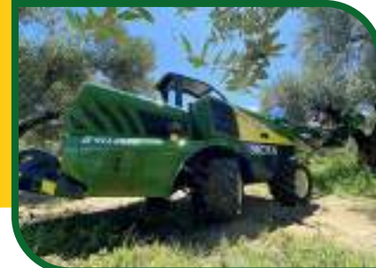
Ponte sterzante posteriore e oscillante Steering and oscillating rear axle
