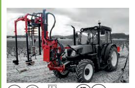
Equipment entirely hydraulic driven (possibility to have different movements simultaneously).
