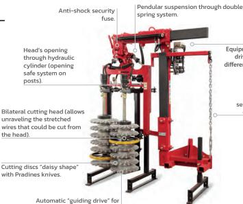
Equipment entirely hydraulic driven (possibility to have different movements simultaneously).
