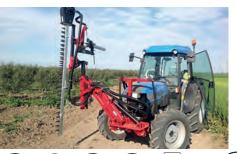
Cutting bars with excentric crankshaft Self-lubricating sliding tray with adjustable nylon rollers. Special steel knives with 4 teeth.
