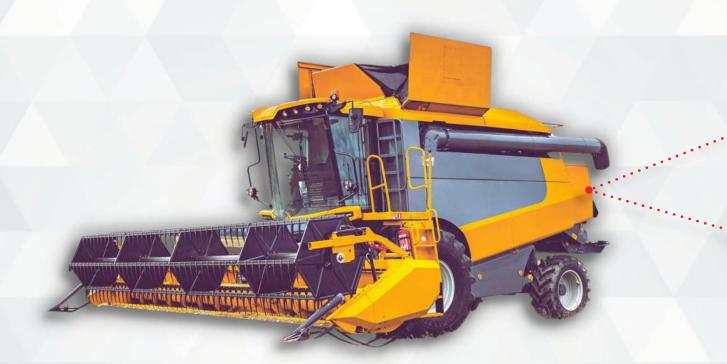
These **high performance sensors** can be mounted on stainless steel bars of various lengths, applicable to all screening and collection systems of the machine and easily installed, tightening the 4 rubber shock-absorbers.
