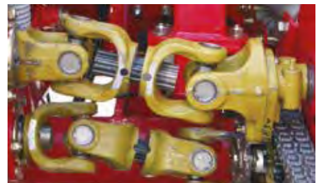
Drive shaft driven feed intake
