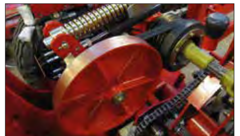
Reverse system is activated from the cabin.
