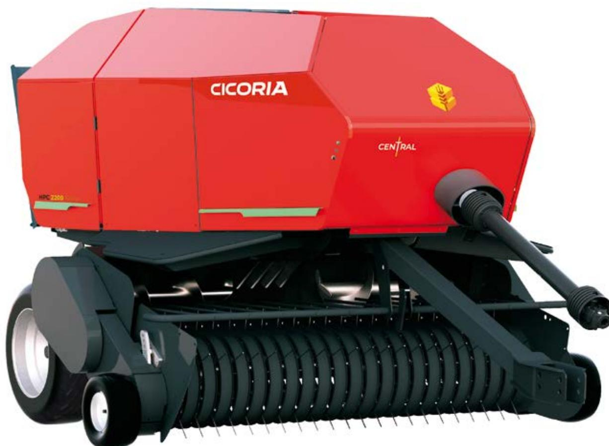
**DESIGN DISTINTIVO AD ALTA EFFICIENZA OPERATIVA, SUPERMANOVRABILE E VERSATILE, MA SOPRATTUTTO PERFORMANTE IN CAMPO, GRAZIE AL PICK-UP ULTRA LARGO E AL PISTONE VELOCE E POTENTE DA 100 COLPI, DOTATO DI ESCLUSIVA CORSA MAGGIORATA PER IMBALLARE AD ALTA DENSITÀ ANCHE I PRODOTTI PIÙ DIFFICILI.**
