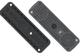
ND emitters eliminate drainage and refill effect, and improve efficiency in pulse irrigation. In order to achieve the Non-Drain function, the emitter closes when the pressure is below 0,1 bar.
