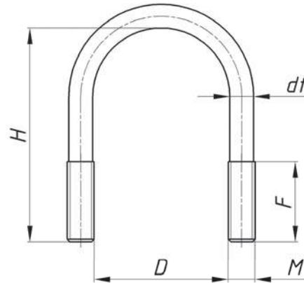
Special U-shaped threaded screw. Suitable for clamping circular section elements of various sizes, from small diameter tubes to big pipes.
