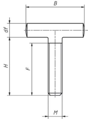
**Cold-pressed part mainly used to obtain an articulated mounting system. Commonly used for mounting tanks.**
