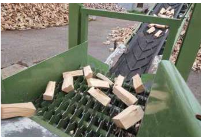
Cleaning rollers for bark and residual sawdust
