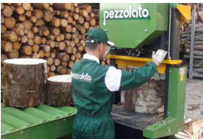
Double manual hydraulic control for wood splitter Wedge
