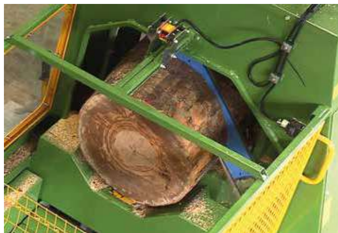
Photocell for automatic log length measurement
