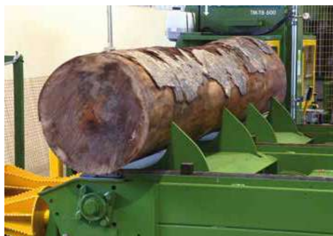
3-chain loading deck, 4 meters in length
