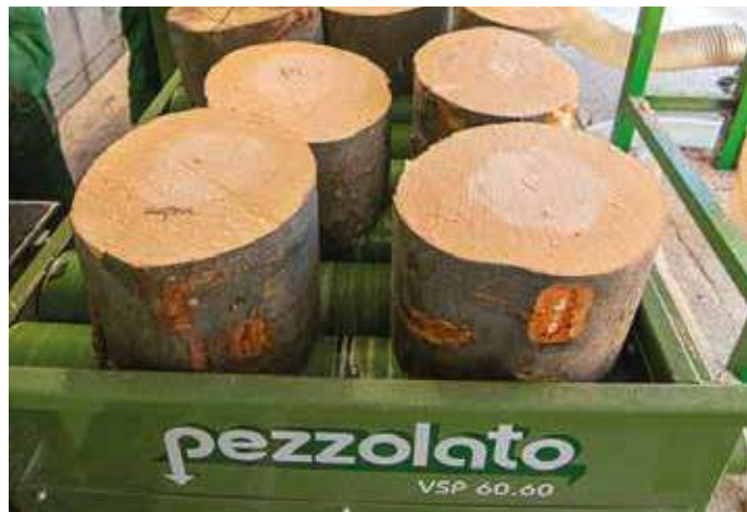
Motorized rollers table for transferring cut logs
