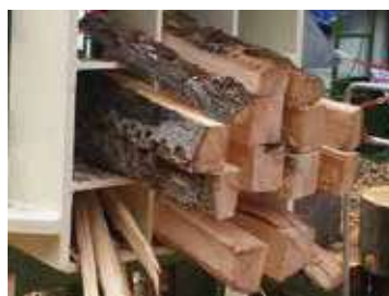
GENIUS WEDGE splitting grid designed to obtain the firewood calibration in one single step, optimising logs diameter and minimising waste
