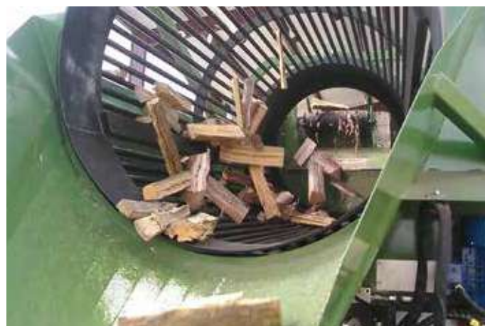
Drum screener for bark and residual sawdust
