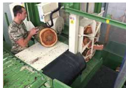
20 Ton splitting station, 2+4+6 folds grid
