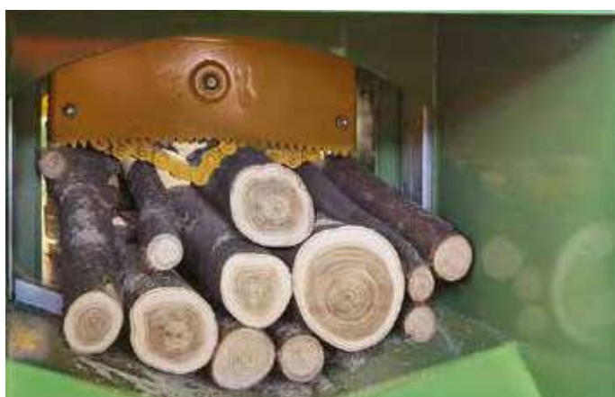
Chain locking system. Efficient on all species of bundles
