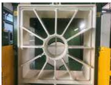
Removable for maintenance operations and interchangeable splitting sector with 10 or 12 or 16 or 18 or 24 folds
