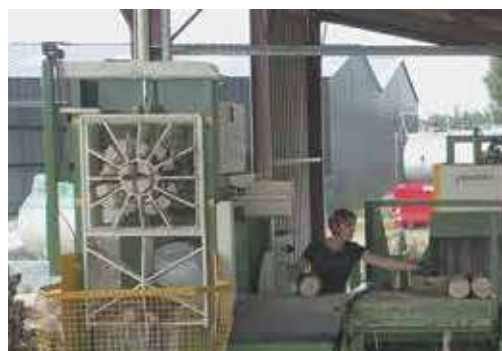
32 Ton splitting station, 2+4+6+16 folds grid
