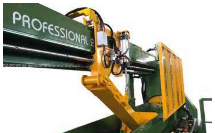
Lifting pusher with mechanical/pneumatic system
