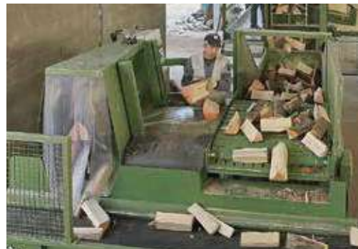
11 Ton splitting station, 2+4 folds grid
