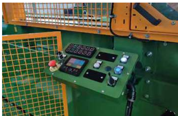
TL 650 - Control panel
