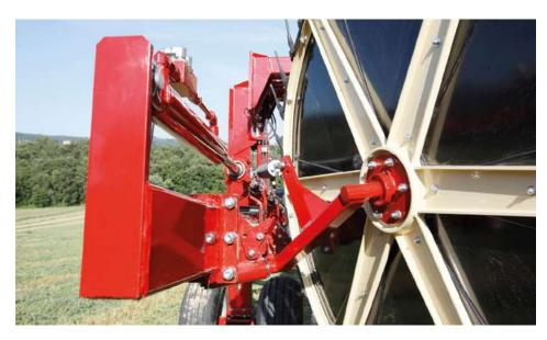
A stop with a safety bolt attached to the sections at each rake wheel lifting arm ensures the stability of the rake wheels during transport. This system also protects the rake wheel lifting arms from accidental knocks and blows while working, since it has been dimensioned so that the safety bolt
