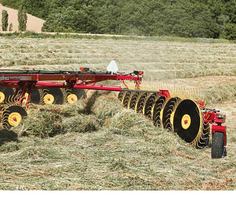
The standard version has rake wheels with a diameter of 55" (1.4m) and tubs with a diameter of 0.28" (7mm). As an alternative, and with no changes to the machine structure needed, it is possible to mount optional rake wheels with a diameter of 60"(1.52m) and tines with a diameter of 0.3" (7.5 mm). Each wheel, regardless of the diameter, is equipped with 40 vats made of top-quality spring steel.
