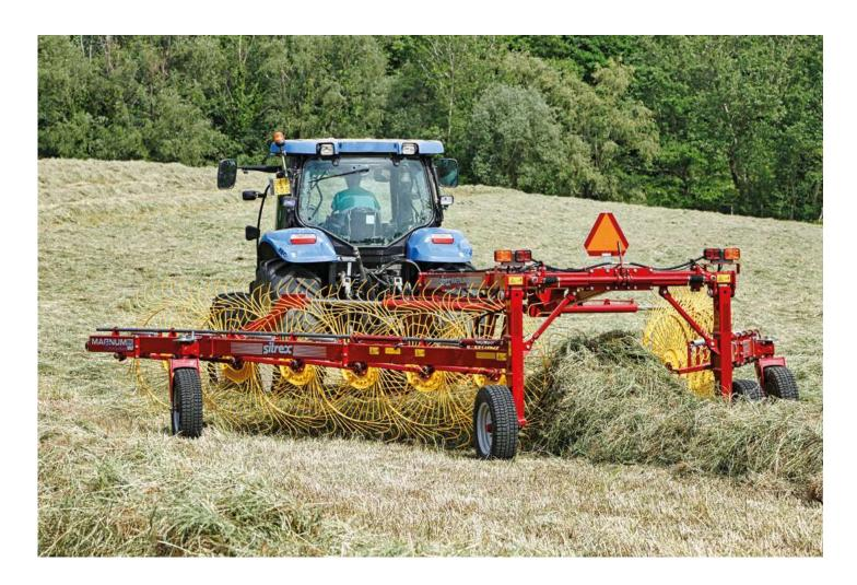
In order to adapt to extreme field conditions, there are rakes that must be solid and sturdy. This is why the drawbar and the rake wings have been made using a large framework of structural tubing to make them tough and fully reliable over time, however hard they are made to work. Despite their size, these machines are easy to handle and transport and very user-friendly.
