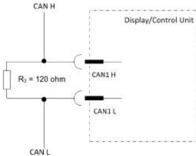
**Example 1.** The figure shows a connection example of an external termination resistor in CAN1
