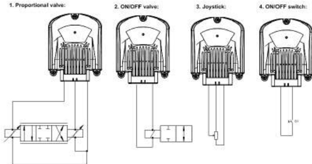
The following figure describes three different ways to connect open circuit loop (from the control unit's point of view):
