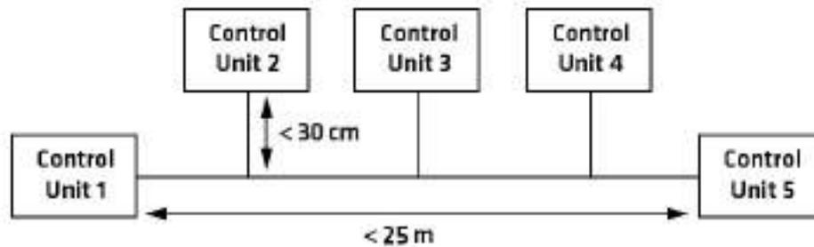
**Example 2.** Control system topology in theory with maximum bus speed (1000 kbit/s); Control Units in traditional bus arrangement. Termination resistor must be connected at control unit 1 and control unit 5. For more information about the bus speeds, refer to CiA DS-102 standard.
