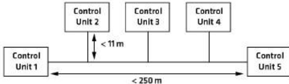
**Example 3.** Control system topology in theory with 250 kbit/s bus speed; Control Units in traditional bus arrangement. Termination resistor must be connected at control unit 1 and control unit 5. For more information about the bus speeds, refer to CiA DS-102 standard.
